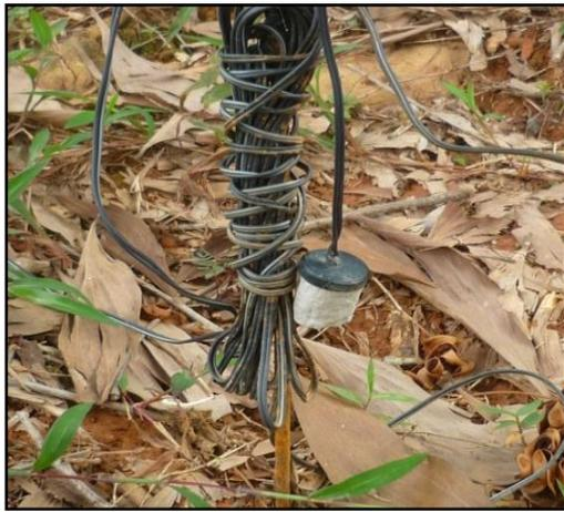
Figure 3 Gypsum block installed at the study area
