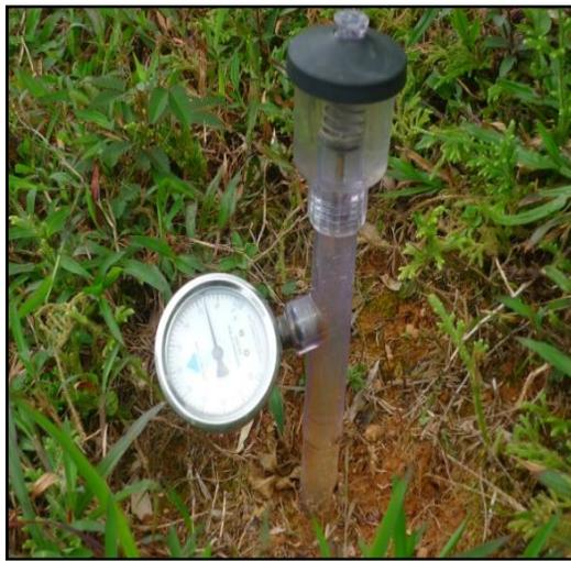
Figure 4 Tensiometer installed at study area
