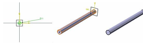
Figure 7 Creation of a circular section strut
